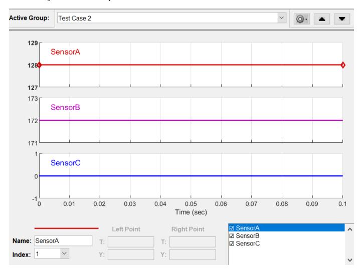
When the input value of SensorA is 128 and SensorB is 172, the Sum block output overflows. The accumulator data type of the Sum block is set to an incorrect integer value of uint8, it results in overflow errors and division by zero errors on the downstream Divide block.
