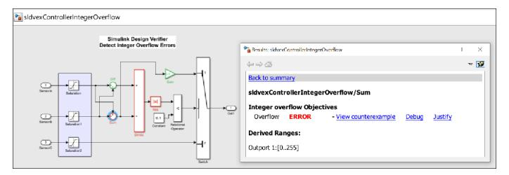
2. To debug the integer overflow error, click **View counterexample**. The harness model and the Signal Builder block open.
